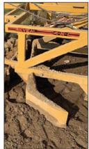
Figure 20. Box scraper, plated, part of multi-unit drag.
