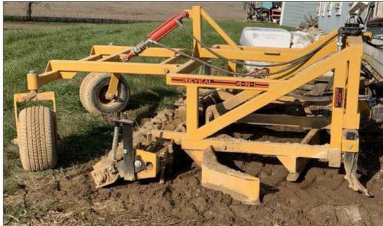
Figure 2. A multi-unit drag can be used for redistributing footing. Claire Burnham, taken at Carriage Station Farm.
