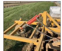
Figure 6. Stroke-control spacer.
