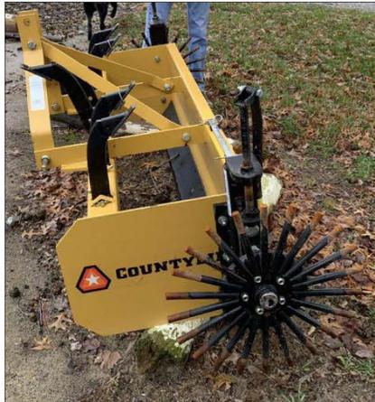
Figure 3. A box grader used to redistribute footing.
