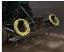
Figure 22. Sawtooth rake with weights.
