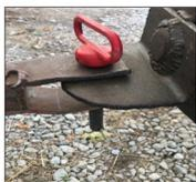
Figure 35. Draw bar attachment with hitch pin connection.
