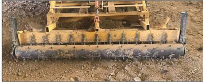
Figure 15. Sheepsfoot roller, part of a multi-unit drag.
