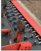
Figure 16. Sheepsfoot roller, part of a multi-unit drag.
