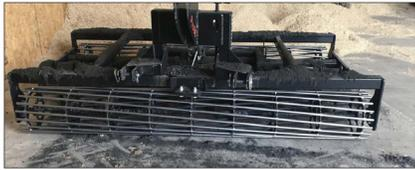
Figure 14. Conditioner, part of a multi-unit drag.
